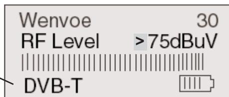
If the meter locks onto a digital carrier DVB-T is displayed and the sounder changes pitch to indicate this.
