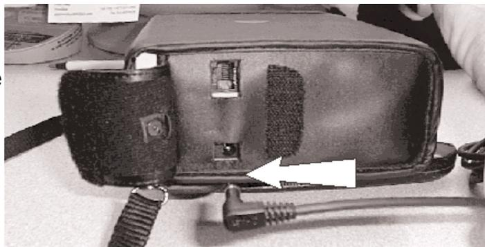
The HDTMv2 can remain connected to either power source, in a "Trickle Charge" state, for an extended period of time without damaging any internal components or the battery pack.
