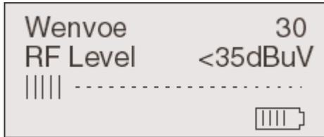
The meter can measure RF level (both analogue and digital channels). BER (Bit Error Rate) in bargraph form for Pre BER and in numerical value for post VITERBI BER. BER can only be measured on digital channels.
